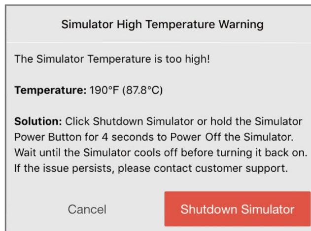
Figure 54: The Simulator High Temperature Warning
